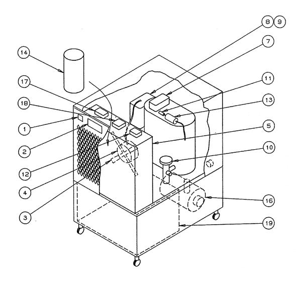
FIGURE 1. CH550 AND CH551 EXPLODED VIEW
